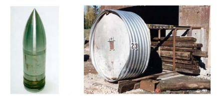
**Fig. 3** The Steel Projectile, Concrete Target used for the Benchmark Test [6]. 11/22
