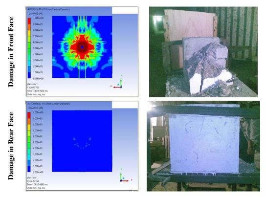
Fig. (8) Front and Rear Damage for Concrete Model SC1
