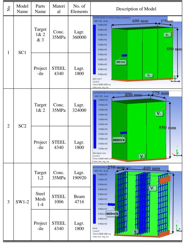
Table (2) The Geometry of Model Parts
