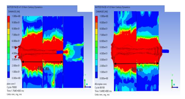
Fig.(4)Depth of Penetration for Model SC1
