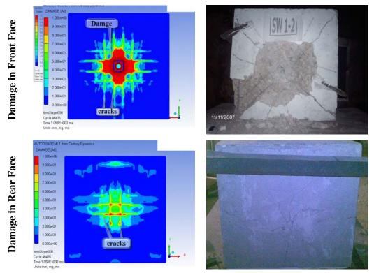
Fig. (10) Front and Rear Damage for Concrete Model SW1-1
