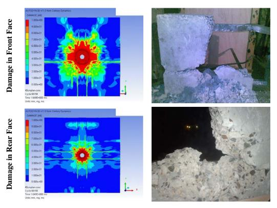
Fig. (9) Front and Rear Damage for Concrete Model SC1
