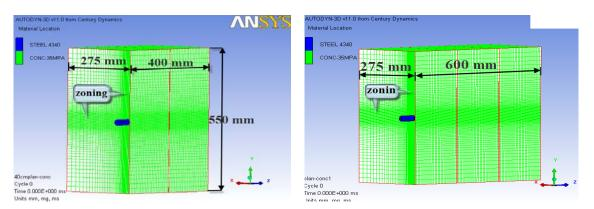
Fig. (2) Geometry and Meshing of the Model SC1 & SC2
