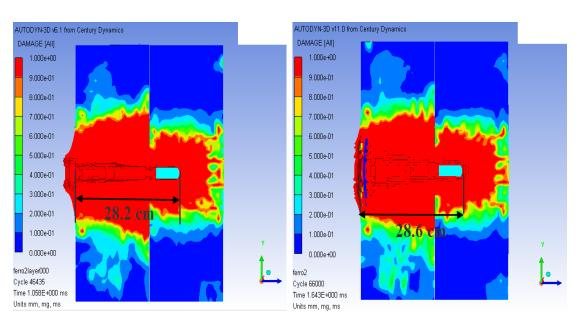
Fig.(6) Depth of Penetration for Model SW 1-2
