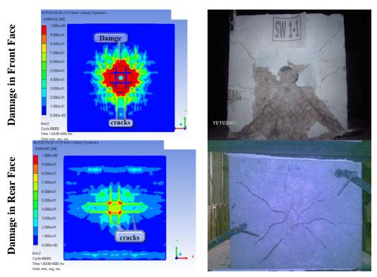
Fig. (11) Front and Rear Damage for Concrete Model SW1-2
