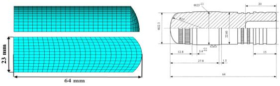
Fig. (1) Geometry and Meshing of the Projectile Part
