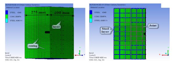
Fig. (3) Geometry , Meshing and Joining of the Model SW1-1 & SW1-2
