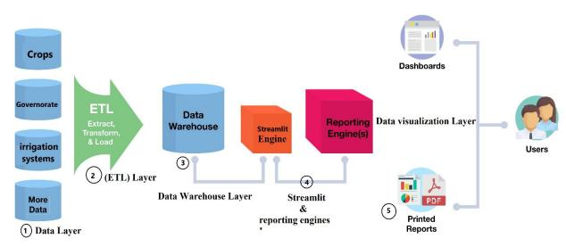
Figure 2 Irrigation systems /BI framework
