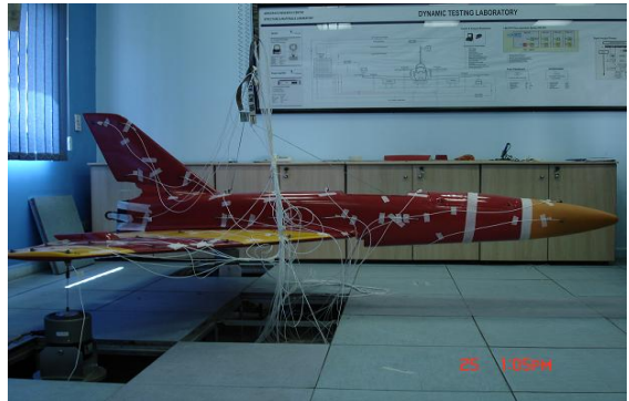
Fig.5.SAHM UAV softly suspended on air-cables
