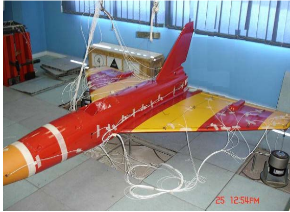
Fig.2. Measurement locations on wing Fig.3. Measurement locations on airframe
