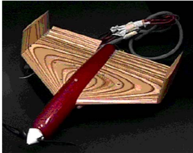
Fig. 3. Experimental model for wind tunnel testing.
