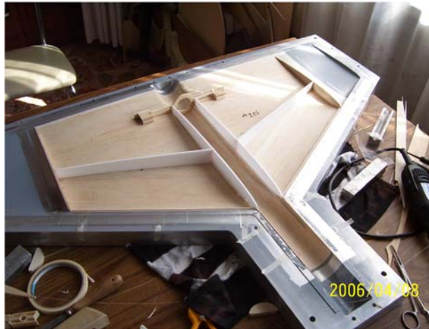
Fig. 7. Production of the airframe (MH600 version).
