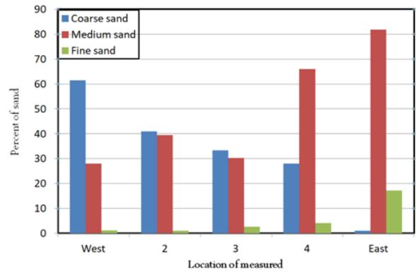
FIG 8. Grain size distribution at c.s 2
