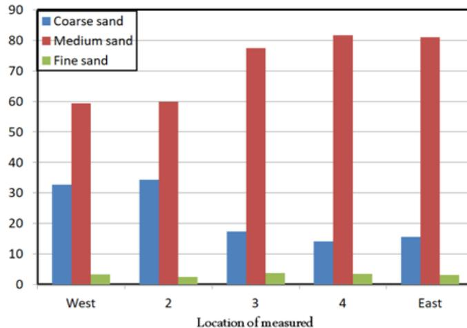
FIG 11. Grain size distribution at c.s 5
