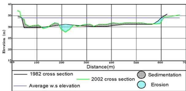
**FIG 14.** The deposition and scour at c.s.1
