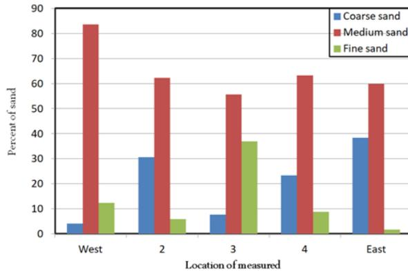
FIG 7. Grain size distribution at c.s 1
