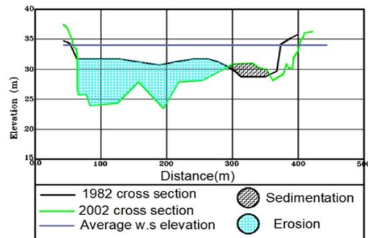
**FIG 15.** The deposition and scour at c.s.4
