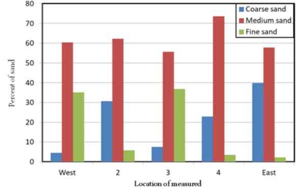
FIG 10. Grain size distribution at c.s 4
