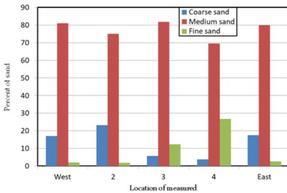
FIG 9. Grain size distribution at c.s 3
