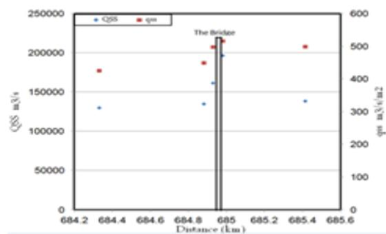
FIG 13. Total suspended sediment and suspended sediment concentration/m<sup>2</sup> at each cross-section
