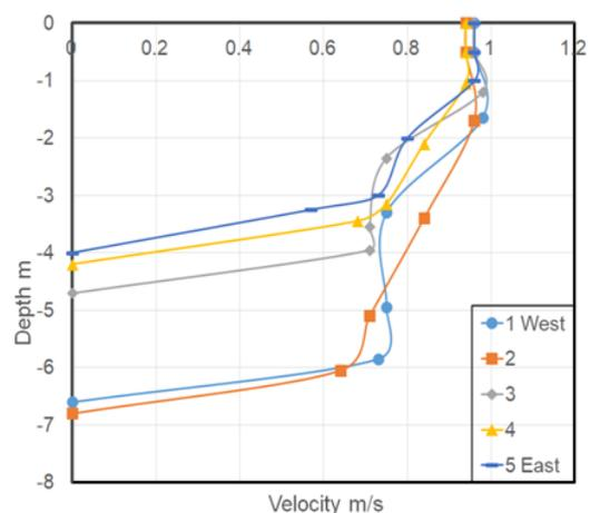
FIG 5. Velocities at cross-section 4
