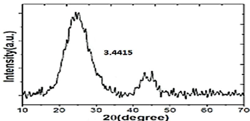
[FIGURE 3]: Identification of carbon ink by X-ray diffraction (XRD) of the paper archive.
