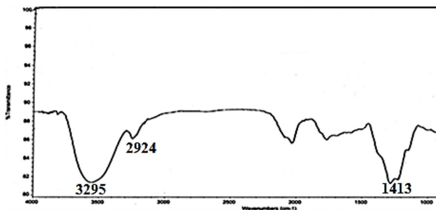
[FIGURE 6]: Fourier Transform Infrared Spectroscopy (FTIR) for determining the ink binder
