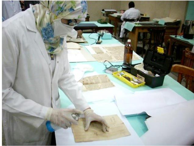
[FIGURE 9]: The disinfection process applied by spray techniques.
