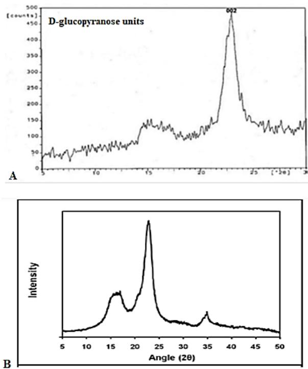
[FIGURE 4]: A- X-ray diffraction pattern of archaeological archive paper (done by researcher) compared to B- the standard X-ray diffraction spectra of cellulose crystallinity<sup>10</sup>
