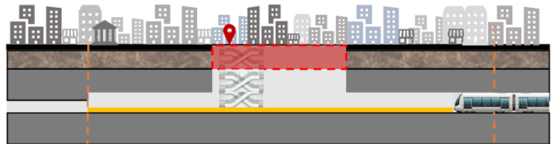
Fig. 12: Cross-section passing through the metro station showing the excavation part in red color.
