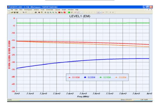
Fig.2. Electromagnetic Simulation Results of the two-way Power Divider
