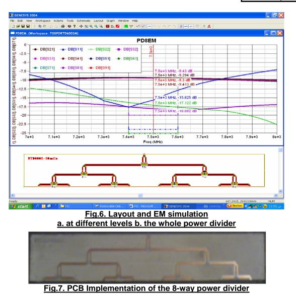
A big enhancement can be observed in the performance of each divider level. Moreover, we can clearly recognize that the overall performance of the divider became much better due to the independent optimizations on the three levels. A perfect matching between each two subsequent stages was achieved and both  $s_{11}$  and  $s_{22}$  became better than -30 [dB]. Even the isolation between two subsequent
