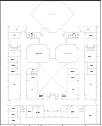
Figure 1. Ground floor plan – engineering university
