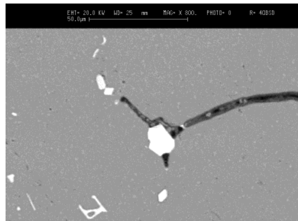
Fig.7. Crack initiation at the triple point occupied with the transforming intermetallic particles.
