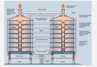
Fig. 17- Eastgate center section Source: <u>https://www.mickpearce.com/</u> <u>biomimicry.html</u>
