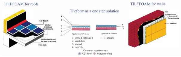
Fig. 13. Tile foam insulation boards layers (13)
