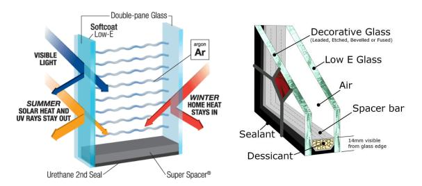
Fig. 12. Double glazed window section (13)
