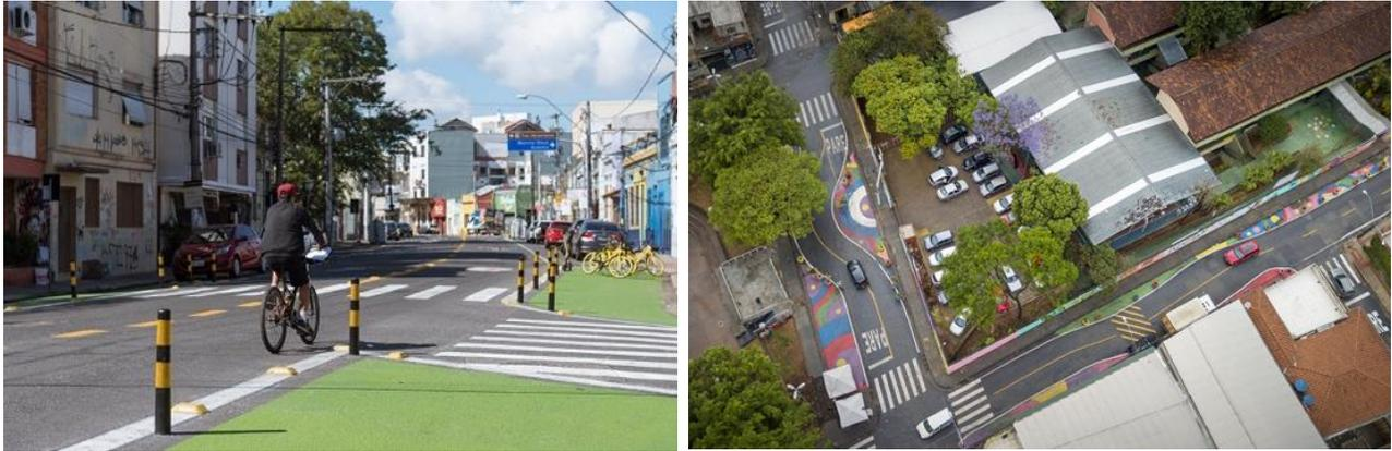
Figure 4: Painted sidewalk extensions and bollards to improve safety for cyclists in painted sidewalk extensions and bollards to improve safety for cyclists. Source: Santos P. M. D., et al., 2020.
