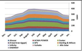
**Fig.10.**Monthly estimation of output of solar energy in benban PV solar park in 2020/2021 by developer
