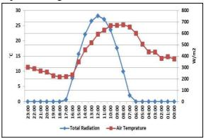
**Fig.14.** hourly relationship between total radiation and air temperature for sun rise company in benban solar park, 31 Dec.2021 Source: author based on sun rise statistics of energy and weather, 31Dec.2021
