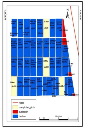
**Fig.8.** layout of benban's PV solar park by developer and capacity, 2022
