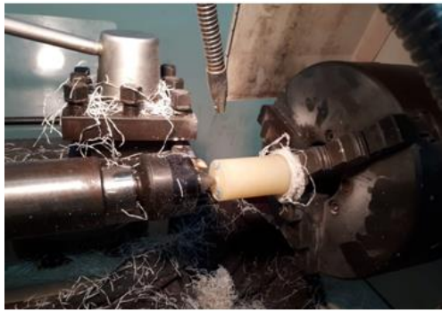
Fig 3. The turning process carried out on epoxy/MWCNTs nanocomposites.
