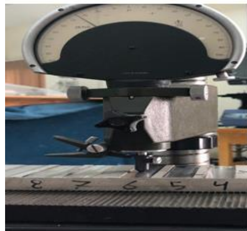
Fig.3 The flatness tester
