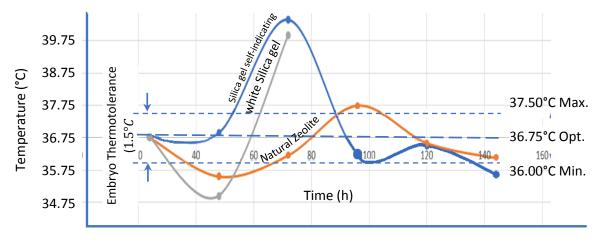
Figure 11. thermotolerance of different TCM battery materials (Silica gel self-indicating, white Silica gel, and Natural Zeolite) during the energy discharging process.
