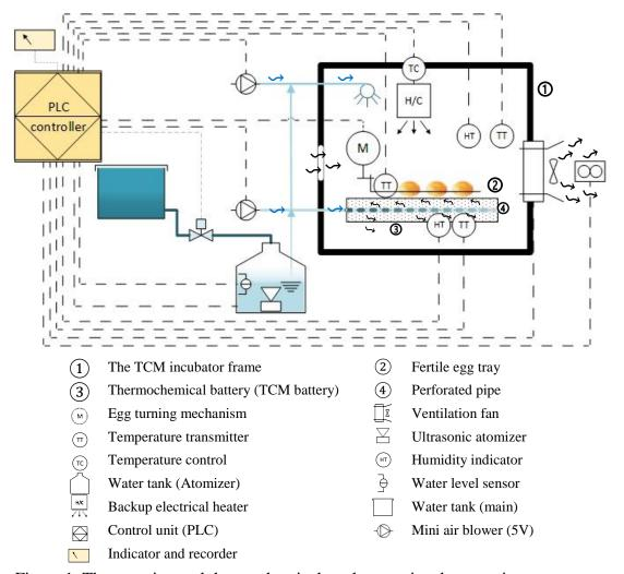
Figure 1. The experimental thermochemical poultry egg incubator main components.
