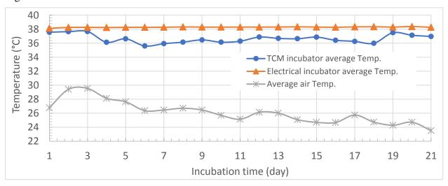
Figure 12. The average atmospheric temperature inside TCM and electrical incubator.
