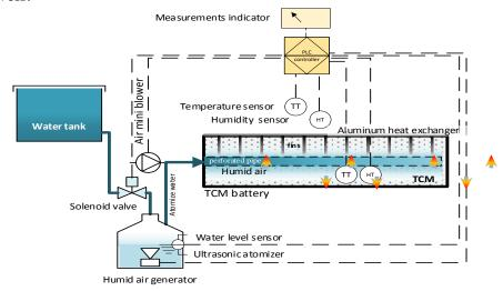
Figure 5. TCM battery discharging process and measurement.
