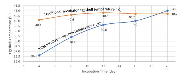
Figure 16. Relationship between average eggshell temperature in the TCM and the electrical egg incubator.
