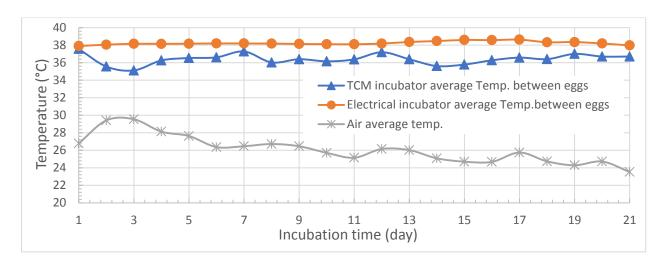
Figure 13. The average temperature between eggs in TCM and traditional incubator
