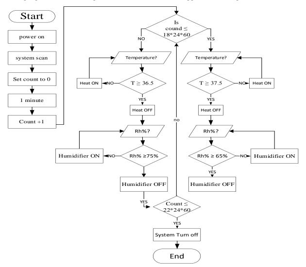
Figure 6. Flowchart of the temperature and humidity control inside TCM egg incubator.
