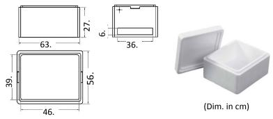
Figure 2. The TCM incubator frame (Styrofoam container).
