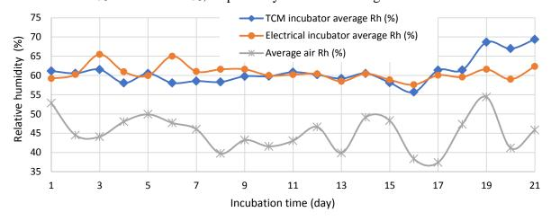
Figure 14. The average relative humidity inside TCM and electrical incubator.
