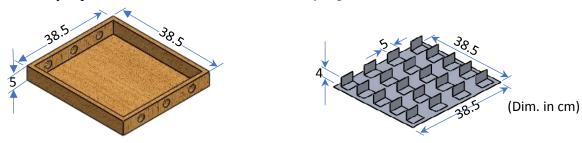
Figure 4. The TCM battery wooden container covered with a finned-aluminum sheet.
