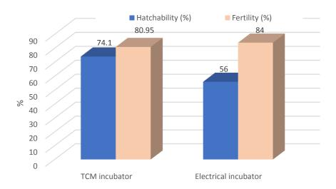
Figure 17. The ratio of hatchability and fertility in TCM and electrical incubator.
