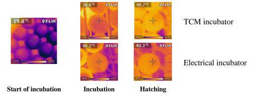
Figure 15. Thermo-image of eggshell at the start, incubation, and hatching stages.
