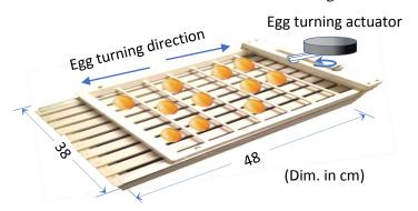
Figure 3. TCM incubator, eggs tray, and turning mechanism.
