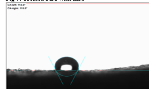
Fig 8: Treated PET/cotton with ZnO
