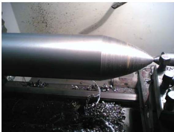
Fig. (2) Manufactured conical nose shape
