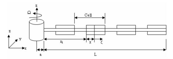
Figure 1: configuration of periodic rotating Timoshenko beam
