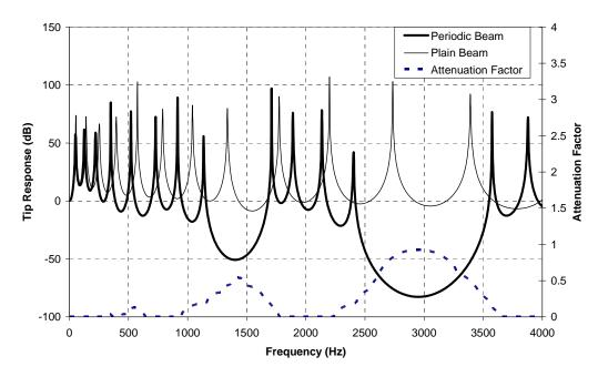
Figure 5: Frequency response of periodic rotating Timoshenko beam (50 rev/sec)
