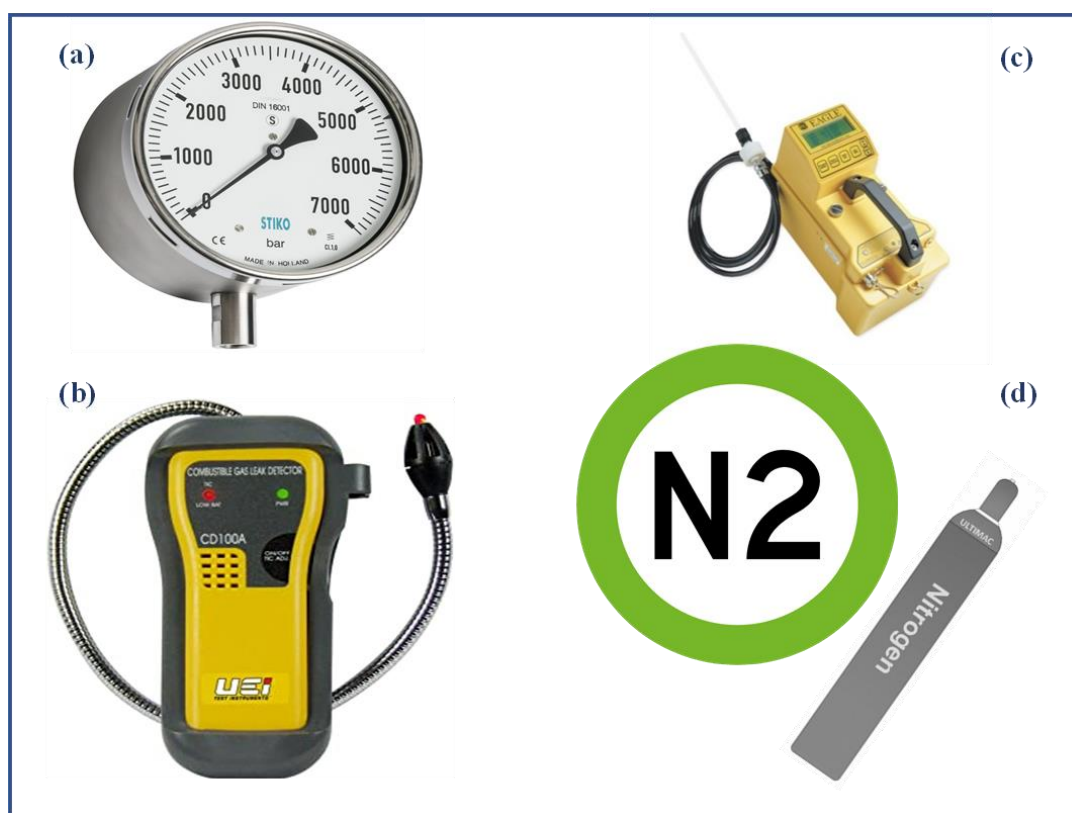
Figure 1. Shows some of the utilized tools during hydrocarbon freeing process; (a) Pressure Gauge, (b) Combustible Gas leak instrument, (c) Mercury test instrument, and (d) Compressed Gas Cylinders ( N_2 ).
