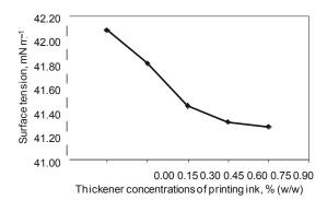
Figure 8: The printing ink's surface tension [17]
