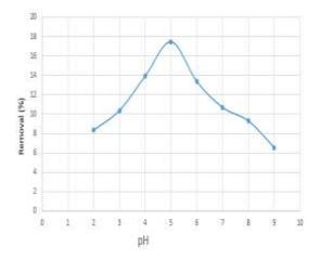
**Fig. (6)** Effect of pH on the removal percentage of methyl orange using the prepared  $Fe_3O_4$ -nps.
