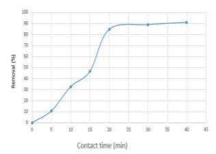
Fig. (4) Effect of contact time on the removal percentage of methyl orange.
