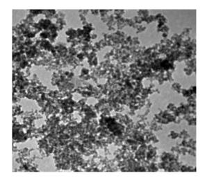
Fig. (2) TEM image for the as-prepared Fe<sub>3</sub>O<sub>4</sub>-nps prepared by the filtrate of A. tamarii.
