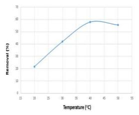
Fig. (8) Effect of reaction temperature on the removal percentage of methyl orange when the experiments conduced with an adsorbent of  $Fe_3O_4$ -nps.
