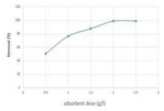
Fig. (5) Effect of adsorbent dosage on the removal percentage of methyl orange using the biosynthetic  $Fe_3O_4$  nps.
