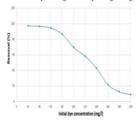
Fig. (7) Effect of initial dye concentration on the removal percentage of methyl orange in the presence of Fe<sub>3</sub>O<sub>4</sub>-nps.
