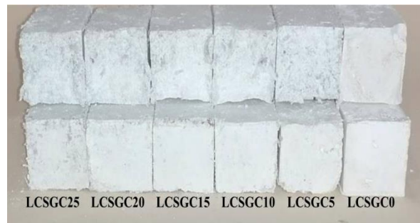
Figure 2. Specimens after the flexural strength test.
