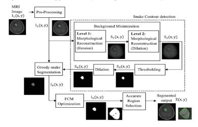
Figure 2: Block diagram of the brain tumor segmentation.
