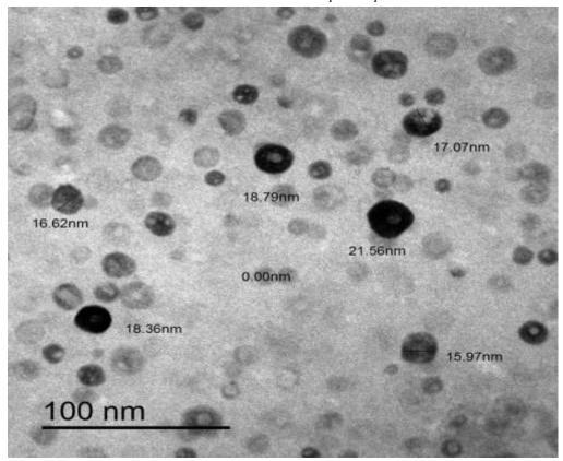
**Figure 1.** The synthesized SeNPs was characterized by transmission electron microscope (type JEOL-JEM 2100). The size of SeNPs arranged between 15.97-21.6nm, with well dispersed and spherical in shape
