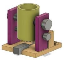
**Figure (3):** Design of the 3D printed custommade device used for air-borne particle abrasion.
