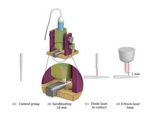
Figure (2): A graphical diagram illustrating the surface treatment applied for each group.
