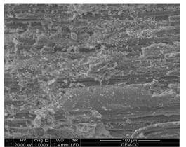
**Figure (12):** SEM micrograph (x1000) of group (D) showing the complete destruction and loss of surface integrity associated with diode laser surface treatment.
