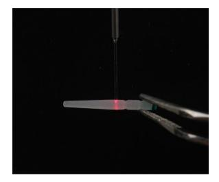
Figure (4): Diode laser irradiation tip applied perpendicularly on post surface in a contact mode.
