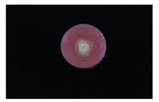
Figure (1): The sectioned tooth inserted in the self-cure acrylic mold.
