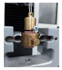
**Figure (7):** The pull-out test using a universal testing machine with the special mandrel attached to the post head.
