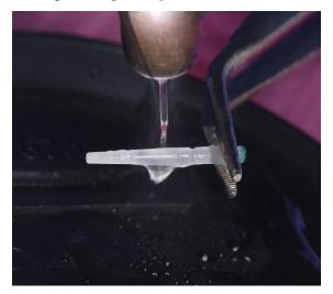
**Figure (5):** Er-Cr:YSGG laser irradiation tip applied on post surface in non-contact mode.
