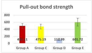
**Figure (8):** Bar chart representing mean and standard deviation values comparing the pullout bond strength with different surface treatments.
