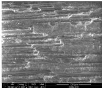
**Figure (11):** SEM micrograph (x1000) of group (A) showing the effect of alumina-oxide air-borne particle abrasion on the surface of glass fiber post.
