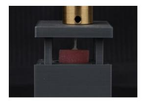
**Figure (6):** Seating of the post under 2.5N axial load using the cementation device.
