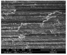
**Figure (10):** SEM micrograph (x1000) of group (C) showing the surface properties of an untreated glass fiber post.
