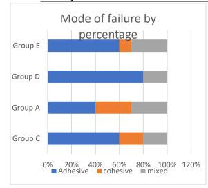
Figure (9): Bar-chart presenting comparing the percentage of different modes of failure for each surface treatment group.
