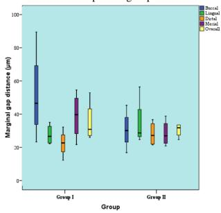
**Figure (8):** Box plot representing median and range values for marginal gap distances in the two groups (Premolar).
