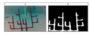
Fig. 12. OpenCV retreived Captured image (A) vs. masked image (B).
