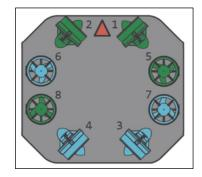
Fig. 1. Our chosen 4x4 thrusters configuration.
