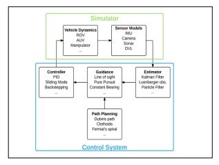
Fig. 8. Block Diagram for software elements.
