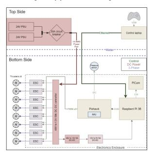
Fig. 4. Electrical circuit diagram of the vehicle.
