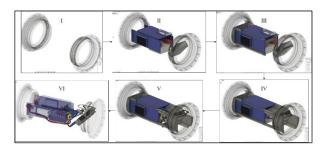
Fig. 6. Design process of first iteration rack. From I to VI: constraints, placement of components in space, sketches and extrusion of the first few 'slices', full design, wiring checks, wiring visible.
