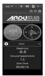
Fig. 11. Representation of pressure, velocity & orientation captured from Ardusub-QGC software.
