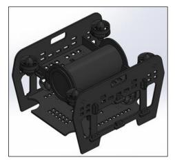
Fig. 2. Complete vehicle assembly in SOLIDWORKS.
