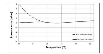
Fig. 10. Pressure error accuracy vs Temperature @850mbar (typical) retrieved from BAR02 datasheet.
