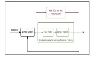
Fig. 9. Data flow diagrams for both simulation and real systems.
