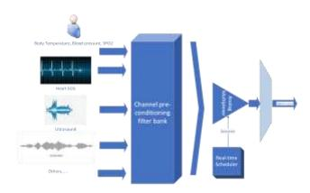
Figure 1: Illustration of a biomedical multichannel heterogenous Data Acquisition with a single A/D converter
