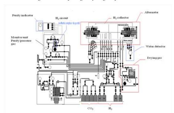
Fig.2. Circuit of the gas hydrogen of the TPP
