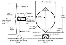
Figure 4 Typical diagram of HAWTs and VAWTs.
