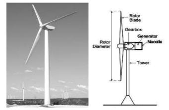
Figure 2 HAWT overview layout (Horizontal Axis)
