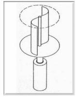
Figure 5 Savonius Wind Turbines
