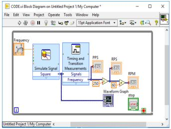
Figure 2.2 block diagram.
