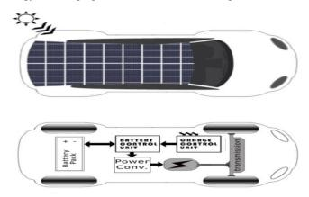
Fig.2 Solar Electric Vehicle drives train with battery pack.
