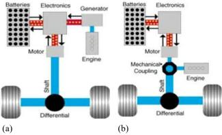
Fig.1 types of hybrid electric vehicles according to way of connection (a) series, (b) parallel.
