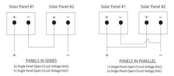
Fig 4: Schematic of two panels in series and parallel.
