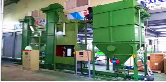
Figure 10. Acid filling machine
