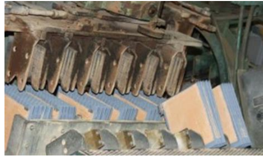
Figure 3. Battery Plates After Pasting and Curing
