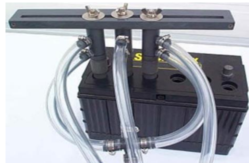
Figure 5. Filling Battery with Electrolyte
