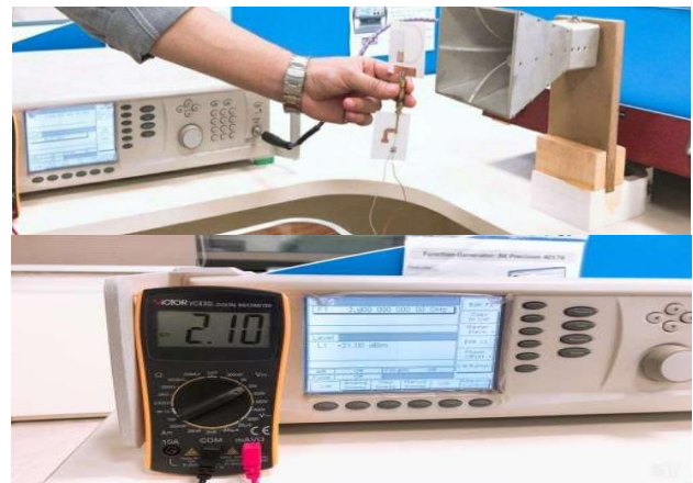
Fig.16 The process of measured rectenna system with monopole antenna
