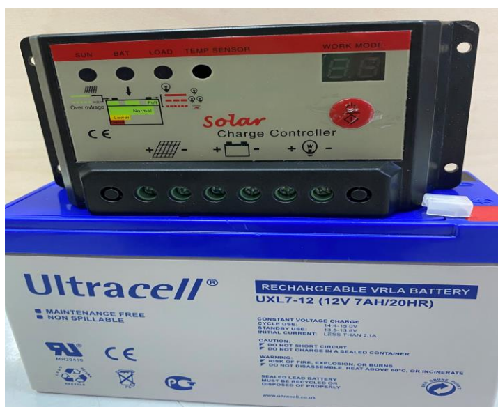
Fig. 15 : Lead-Acid Battery with solar controller.
