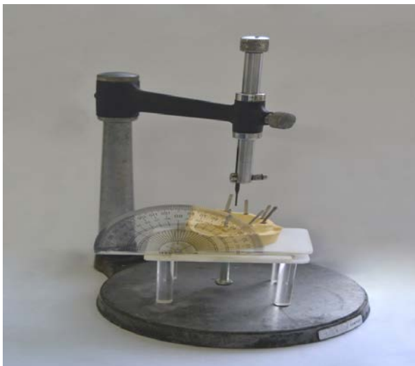
Figure 4. Full measuring apparatus setup. Analyzing rod attached to tool holder.
