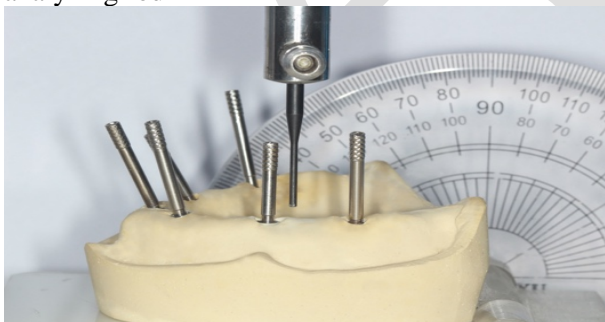
Figure 5. The long axis of the reference implant (R) aligned to be parallel to the analyzing rod
