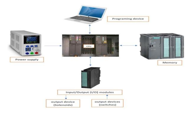
Figure 4: Block diagram of PLC.
