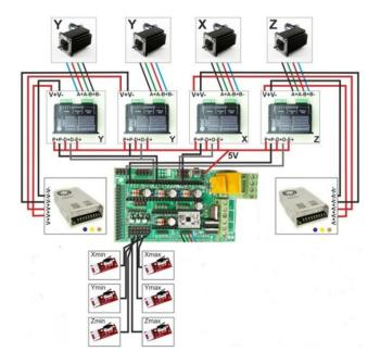
Fig. 2 wiring diagram of the project
