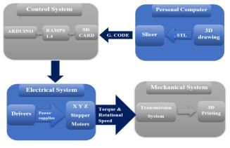
FIG.1 BLOCK DIAGRAM OF PROJECT DESIGN
