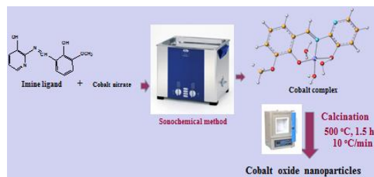
Figure (1) Shows the preparation of \text{Co}_3\text{O}_4 nanoparticles (after, Abdel Rahman, et al, 2017) [22].
