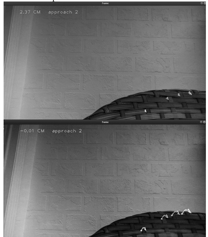
Figure 3: shows the linear odometry by using second method (tracking special color)
