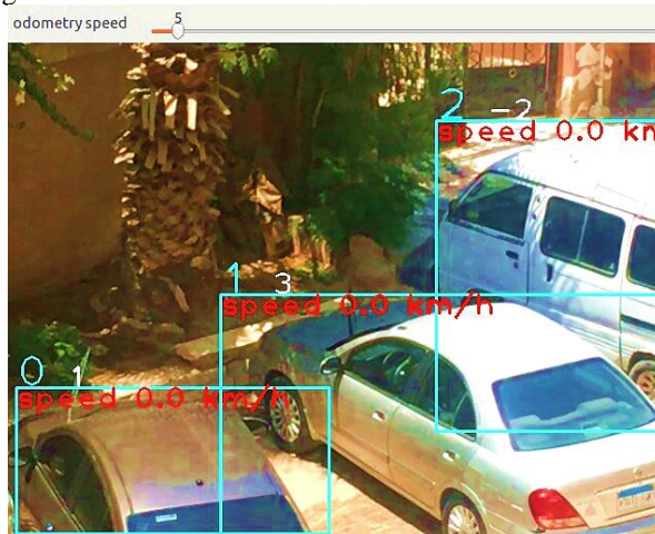
Figure 12: tracking all road cars with a certain ID for each car and calculating the speed for each of them. it shows speed zero because all this car is parking.
