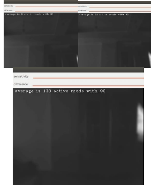
Figure 4: shows the difference (average) between frames in static mode (no change in odometry) and in active mode (change in odometry)
