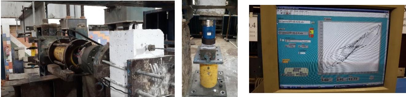
Figure 5: The horizontal-vertical actuator and digital recording computer system
