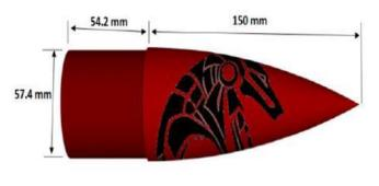
Figure 3 Nose Cone Design [2].
