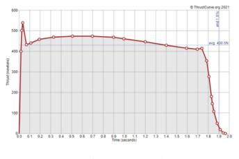
Figure 7 Thrust Time Curve (18A) [4].
