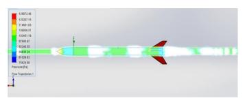
Figure 14 Pressure Distribution Without After Body [8].
