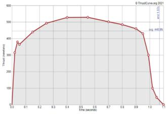
Figure 6 Thrust Time Curve (16A) [4].
