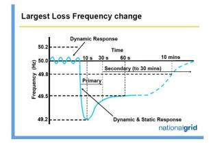
Fig. 6- Primary and secondary frequency responses
