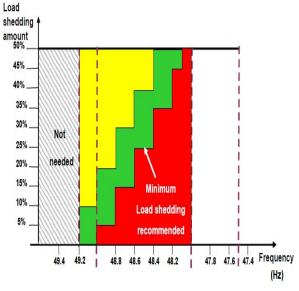
Fig. 5- ENTSO-E recommended UFLS [12]
