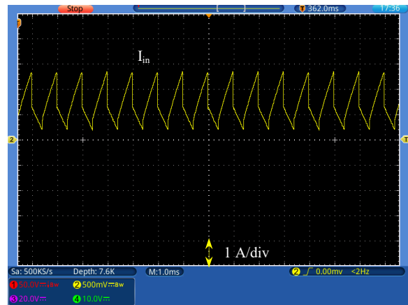
Figure 6- Waveform of input current in CCM
