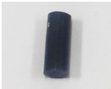
Fig. 4 Sample of PMMA material reinforced with SWCNT.
