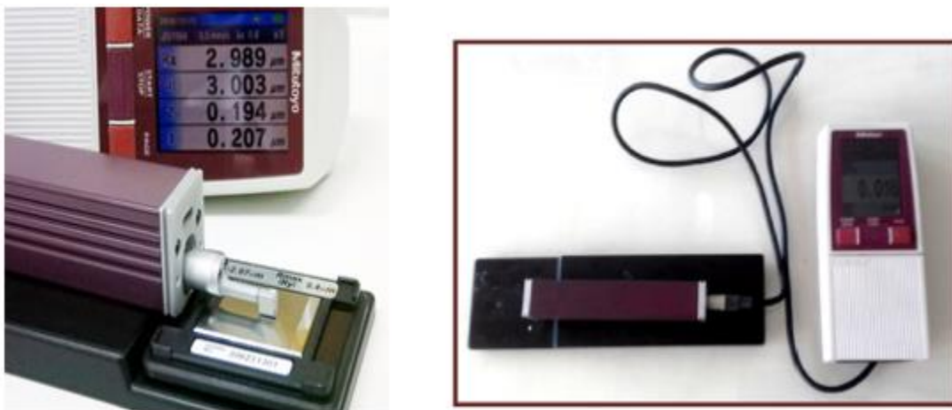
Fig. 6 The surface roughness measuring tester (SJ-210).
