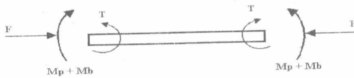
Fig. A2 Loads acting on the frame during operation.
