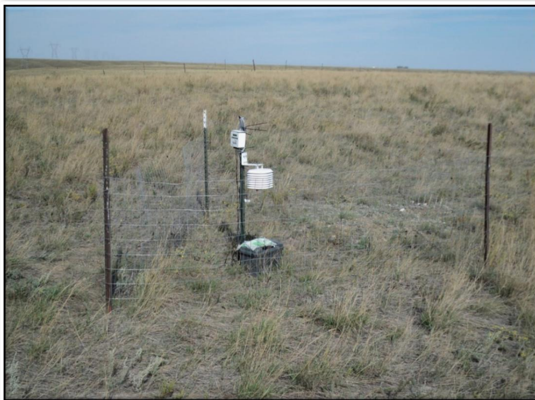
Fig. 5c. Soil moisture and air temperature sensors set up at a study site in Montana, USA. Photo by Brevik
